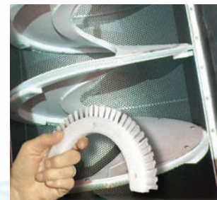
Durable segmented brushes make replacement easy.
