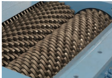
Twin-shaft cutting chamber.
